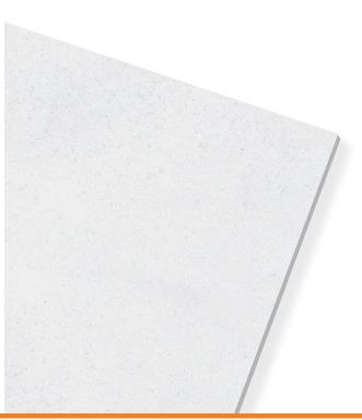
THERMATEX® Acoustic is a 19 mm thick ceiling tile made from a special perforated mineral board with an acoustic fleece facing. The perforations provide excellent sound absorption while the fleece offers a smooth, elegant surface finish. The combination of high density, bio-soluble mineral wool with clay and starch provides excellent physical characteristics, particularly for acoustic performance.
