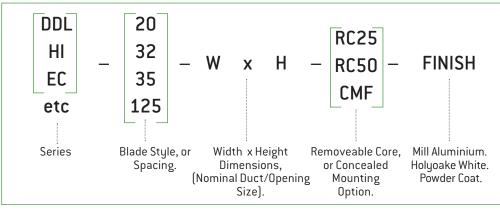
Grilles/Registers shall be of aluminium construction and shall be supplied with the "Holyoake" Removable Core RC System, or Concealed Mounting Frame System, allowing the Grilles/Registers to be easily removed for cleaning, access and maintenance. The removable core subframe shall be an integral part of the Grille/Register.
