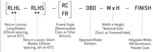
\*\*Suitable for Passive Ventilation (Do not exceed core velocity of 2.5m/sec).
