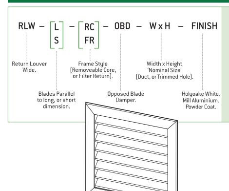
Return and/or exhaust louvers shall be of extruded aluminium, rattle-free construction, of the model shown on the drawings, or elsewhere in this specification. Blades shall be mechanically locked to mullions and frames. Frames shall have close mitred corners, reinforced and secured with aluminium gussets. Filter returns, where specified, shall be of similar construction, mounted in a hinged subframe and held closed with a positive latch. Filters are 'EU2' washable type.
