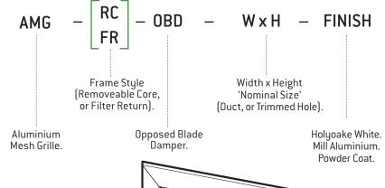
Return and/or exhaust Grilles shall be an aluminium frame with aluminium mesh core. They shall be of rattle-free construction, of the model shown on the drawings, or elsewhere in this specification. Frames shall have close mitred corners, reinforced and secured with aluminium gussets. Filter returns, where specified, shall be of similar construction, mounted in a hinged subframe and held closed with a positive latch. Filters are 'EU2' washable type.
