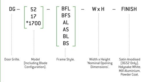
Door grilles shall be of rattle-free, all aluminium construction, with sight proof blades of Chevron design, assembled in either a flanged, or channel type frame, presenting a similar appearance from both sides. Purpose made back flanges shall be available for flanged units, standard models shall be available to suit any door thickness from 28mm to 52mm.
