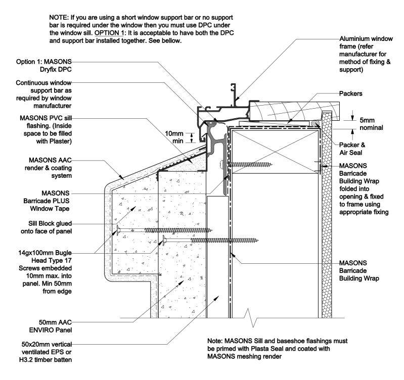
**OPENING FLASHINGS Alternative Window Sill**  Detail 22 Scale 1:2
