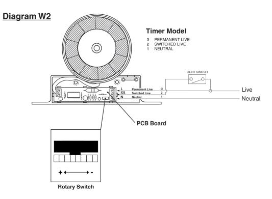
9 Remove the cover on the Fan Bracket and make the electrical connection as follows:
