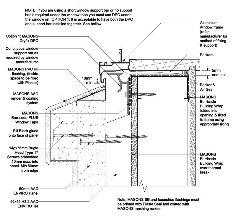
OPENING FLASHINGS **Alternative Window Sill**  Detail 24 Scale 1:2
