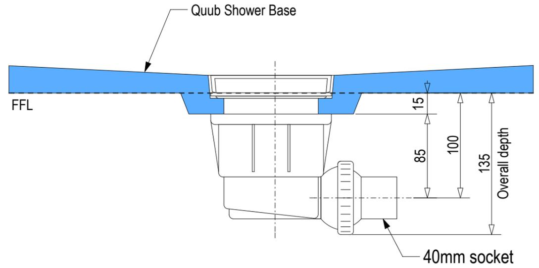
Ensure a minimum recess size of 250mm wide x 250mm long x 150mm deep for the channel drain and waste outlet
