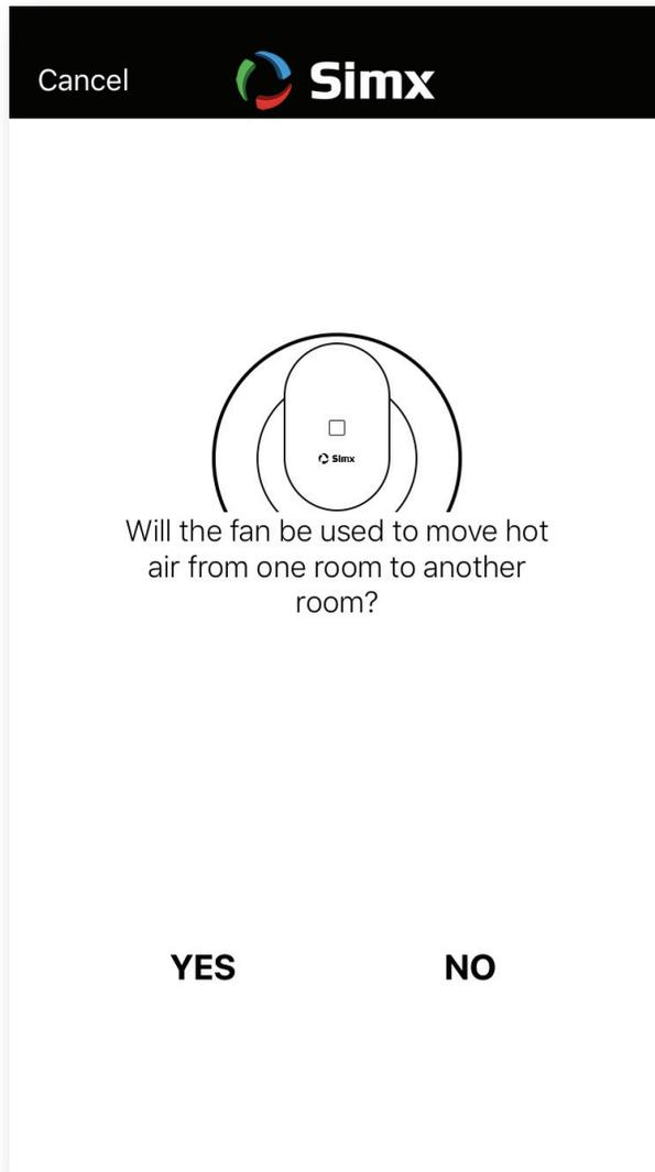
Manrose Genius can be set-up as a Heat Transfer unit to move warm air through an internal wall from one room (eg. lounge) to an adjacent room.
