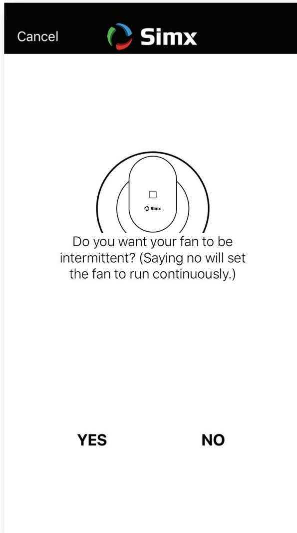
The fan can also be used as an intermittent fan or as a continuously running fan.
