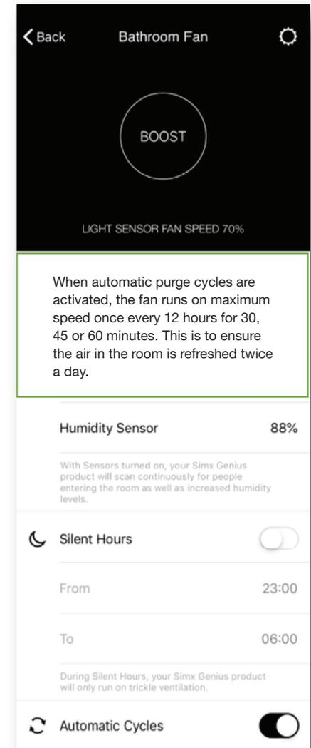
When automatic purge cycles are activated, the fan runs on maximum speed once every 12 hours for 30, 45 or 60 minutes. This is to ensure the air in the room is refreshed twice a day.
