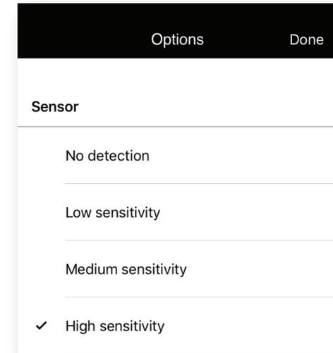
Select sensitivity of the humidity sensor system. This adjusts the rate of humidity change required to trigger the fan. You can then use the sliding scale to increase or decrease the air moved in the function.
