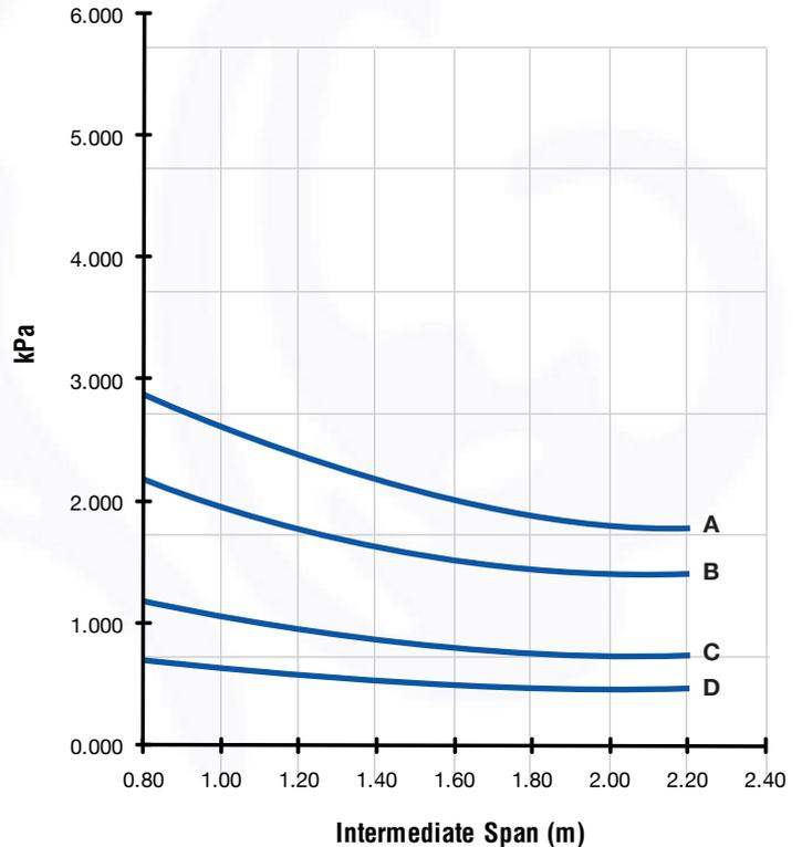
Note: The intermediate spans shown in the graphs above are based on G550 Steel as the base metal. To calculate end spans please multiply the intermediate span calculated by 0.66. Spans are based on restricted access. For alternative metals please contact your local Metalcraft branch.
