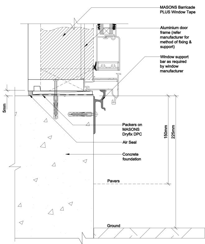
**OPENING FLASHING -CONCRETE DOOR SILL** Without Rebate
