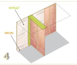
Install the INTELLO membrane on the inside of the external wall and uppermost ceiling, where it meets the INTELLO PLUS connection strip allowing for an overlap of 20 – 30 mm.
