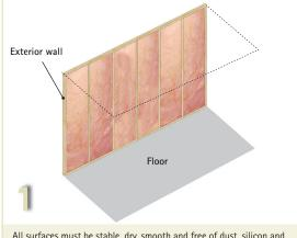
All surfaces must be stable, dry, smooth and free of dust, silicon and grease. Sweep or vacuum clean and wipe all surfaces.
