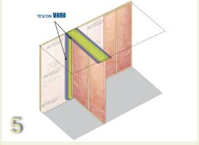
Once all of the INTELLO membrane is installed apply the TESCON VANA multi-purpose adhesive tape to the overlap between the INTELLO membrane and the INTELLO PLUS connection strip to form a continuous airtightness layer.
