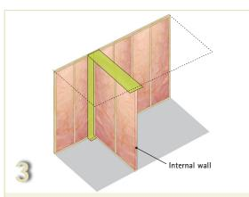
Erect the internal wall allowing an even overhang of the INTELLO Plus connection strip on either side of the internal wall.
