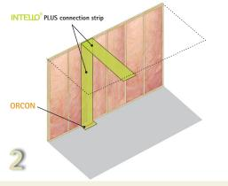
Prior to erecting of the internal wall, fix the INTELLO PLUS connection strip to the junction where the internal wall meets the external wall using stapes at 200 mm centres. Apply the pro clima ORCON multi-purpose joint adhesive to connect the INTELLO PLUS connection strip to the subfloor.
