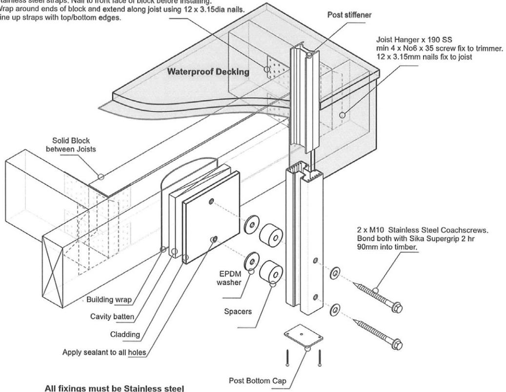
Design engineer must ensure deck can support a moment of 2.03 KNm applied at each post
