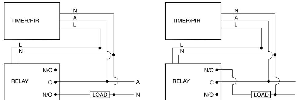
Figure 1: Relay Wiring Diagram
