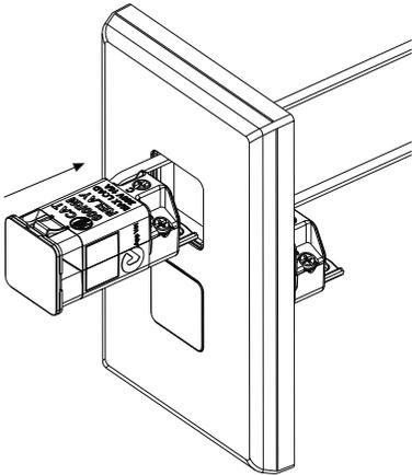
Figure 3: Mounting Relay To Sub Plate
