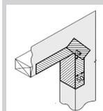
1. Install lintel pieces on top corners of opening, 200mm along the lintel and 200mm down the jamb. Slit at each corner and fold onto outer face of building wrap (at least 50mm).
