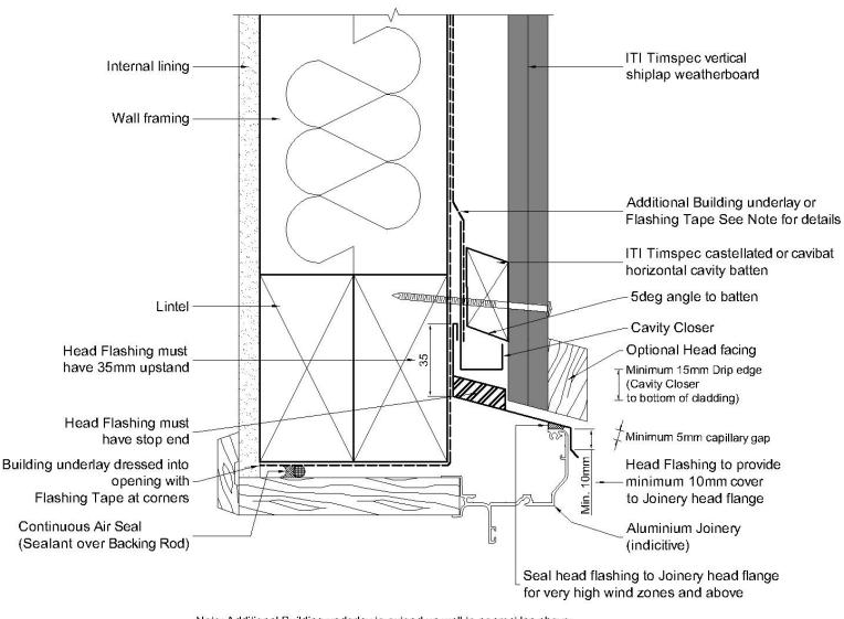
Note: Additional Building underlay to extend up wall to nearest lap above and extend down as far as possible into Cavity Closer. Alternatively Elashing Tane to extend up wall a minimum of 50mm above Cavity
