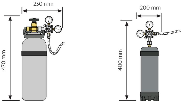
Secure cylinder vertically to a robust surface with the hook & loop strap and bracket supplied.
