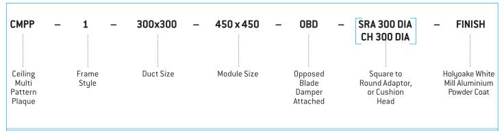
Ceiling Multi Pattern - Plaque Louver Face diffusers shall be type CMPP. They shall be of all Aluminium construction, with removeable plaque core. CMPP have a range of frame styles and accessories for installation and volume control.
