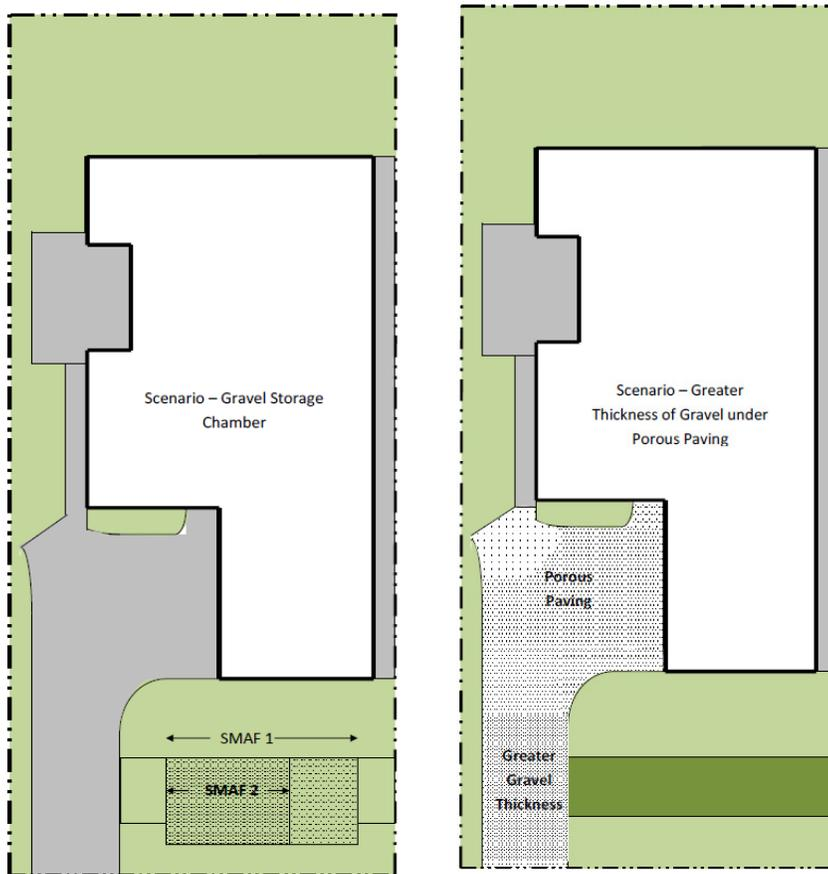
Figure 2-2 Single House Stormwater Management Scenarios (D&B Kettle Consulting Ltd 2013a)
