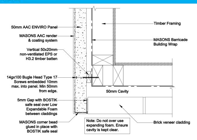
**AAC ENVIRO PANEL / BRICK VENEER** Detail 45 Scale 1:5
