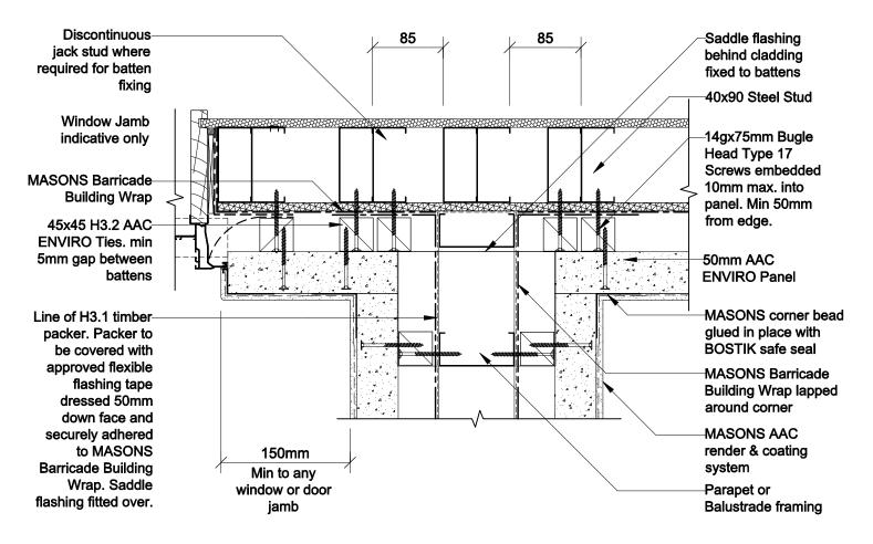
PARAPET / HANDRAIL TO WALL JUNCTION With Metal Capping Detail 57 Scale 1:5
