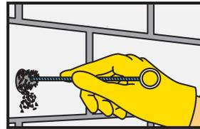
3. The drill hole must be thoroughly cleaned with the special steel brush (brush at least 2x). The diameter of the brush must be larger than the diameter of the drill hole
