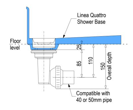
Ensure a minimum recess size of 150mm wide x 600mm long x 150mm deep for the channel drain and waste outlet
