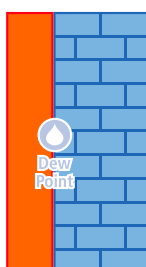
Internal wall insulation
