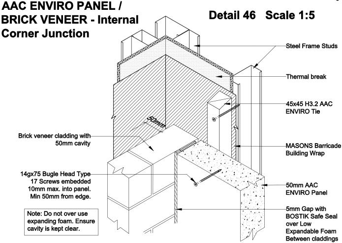
**AAC ENVIRO PANEL / BRICK VENEER Internal Corner Junction - 3D View**
