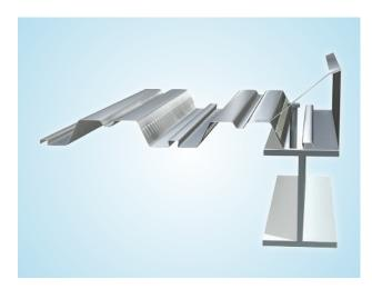
Figure 3: Typical edge form layout flush to beam edge
