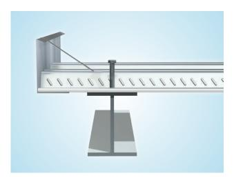
**Figure 4:** Typical edge form profile layout with cantilever – edge form held square with restraint straps
