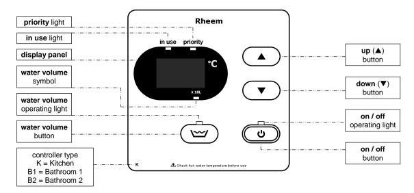
**Note:** water volume () utton, water volume operating light and water volume symbol are on the Kitchen controller only.
