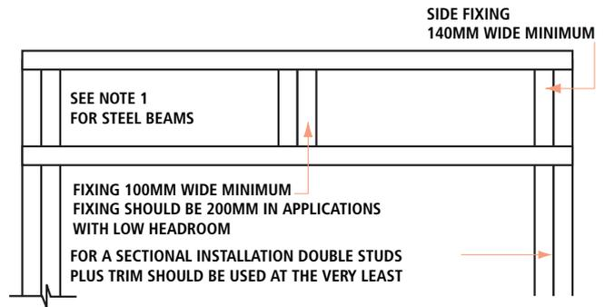
**NOGGING DETAIL FOR SECTIONAL UP TO 2.3M HIGH (TRACK AND MOTOR FIXINGS)**
