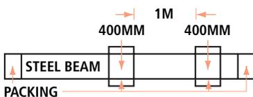
**PACKING FOR STEEL BEAMS ('I' OR 'U' SHAPE)**
