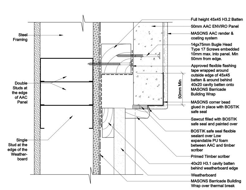
**AAC ENVIRO PANEL / WEATHER BOARD VERTICAL JUNCTION** Detail 42 Scale 1:2 **Plan View**
