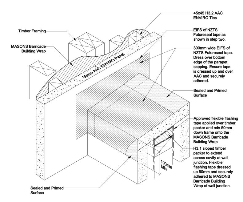
PARAPET / HANDRAIL TO WALL JUNCTION ENVIRO Panel Capping Step 3 **Detail 46B NTS**
