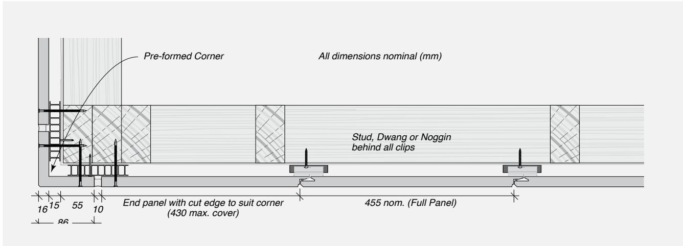
FIGURE 7.05 Typical Framing Set-Out with 70mm Timber Framing and Territory Pre-formed Corners – Plan View
