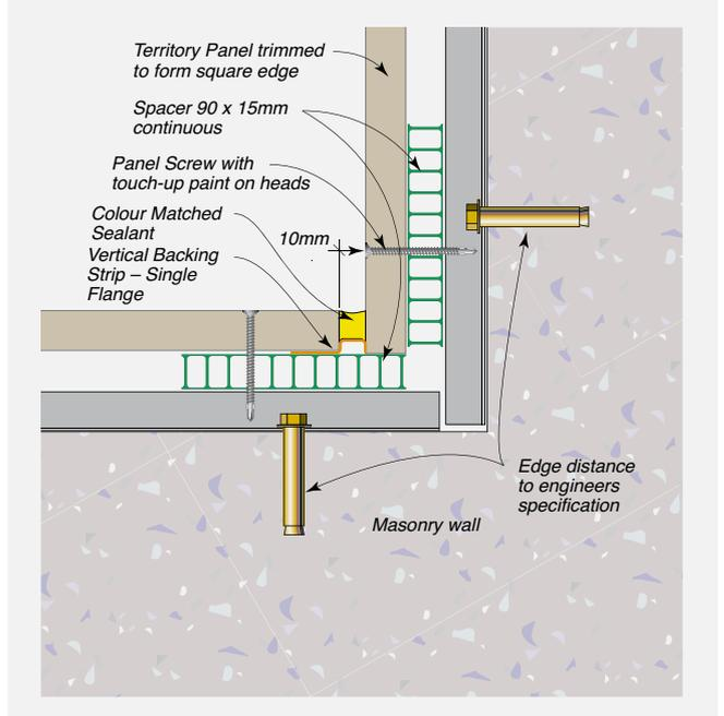
**FIGURE 8.43** External Corner Detail – With Coloured External Corner Trim – Plan View
