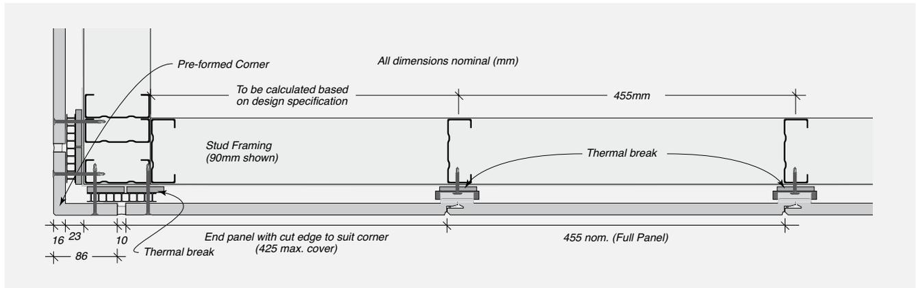
FIGURE 7.09 Typical Framing Set-Out with 75mm Steel Framing and Territory Pre-formed Corners – Plan View
