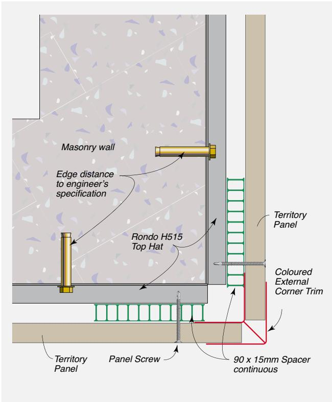
**FIGURE 8.45** Parapet Detail – Elevation
