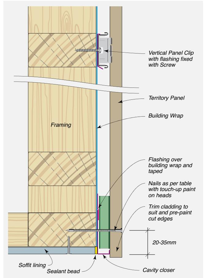
**FIGURE 8.06** Soffit Detail – With Timber Trim – Elevation
