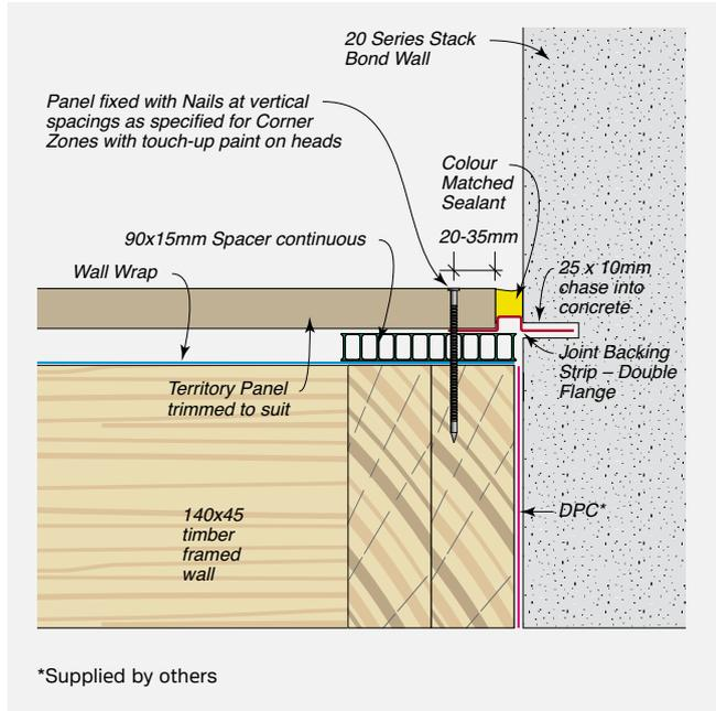
**FIGURE 8.34** Typical Abutment – Panel to Weatherboard – Plan View
