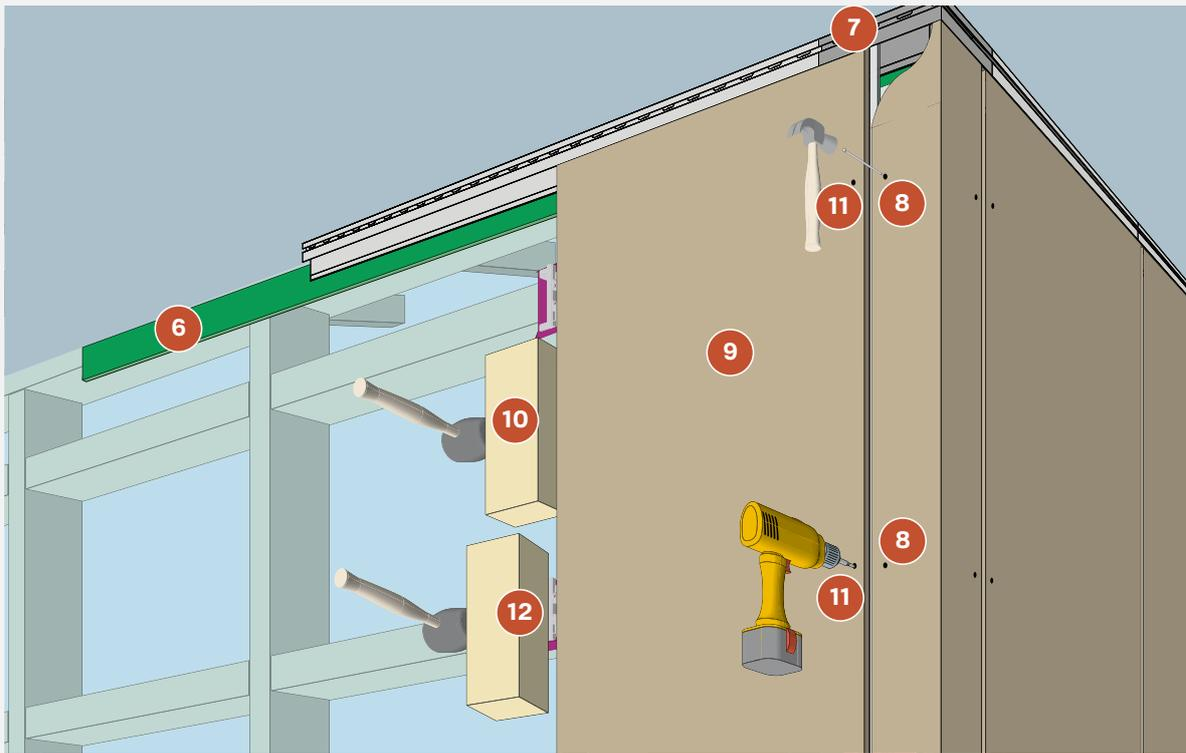
13 Lift the next panel into position, placing the head into the soffit trim and base onto the starter strip. 14 Slide the panel into the existing clips. Firmly tap panel into position. 15 Fit and fix panel clips and panel clip flashings to the framing as for the previous clips. Repeat steps 13, 14 and 15 for additional panels. 16 Mask and prime edges of expressed joint and fill joints with colour matched sealant. Prime and touch-up visible fixing heads.
