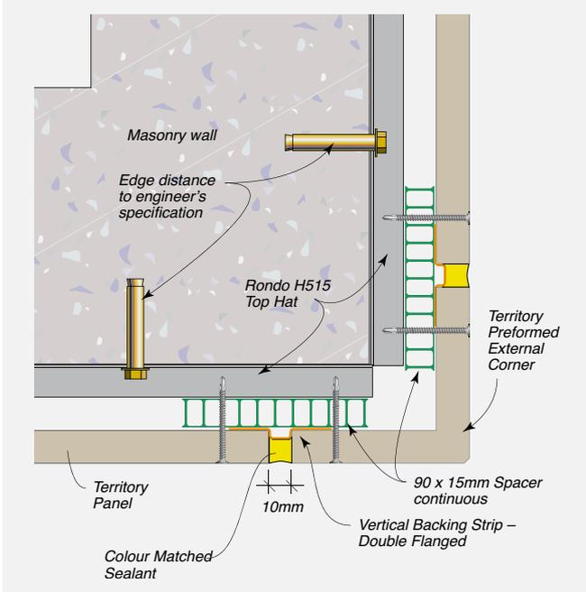
**FIGURE 8.44** Internal Corner Detail – With Backing Strip and Colour Matched Sealant – Plan View
