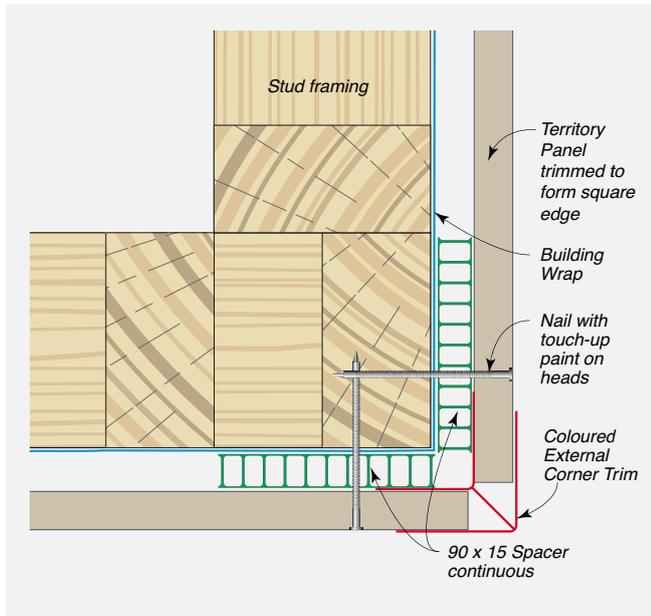
**FIGURE 8.11** Obtuse Angle Corner Detail – With Metal Flashing and Colour Matched Sealant – Plan View
