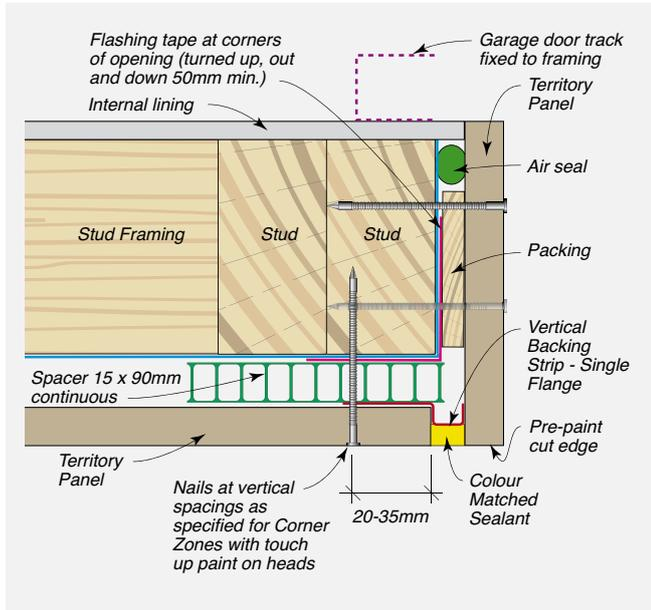
**FIGURE 8.15** Typical Garage Door Head Detail
