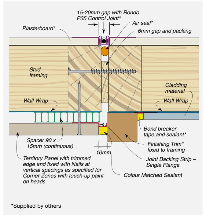
**FIGURE 8.37** Typical Abutment with In-set Masonry Wall – Plan View
