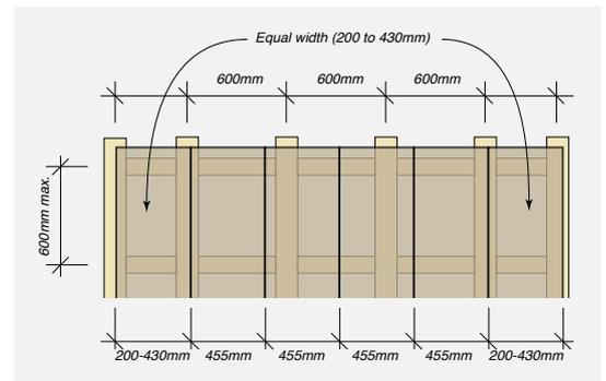
**FIGURE 7.03** Symmetrical Panel Set-out – Steel Framing
