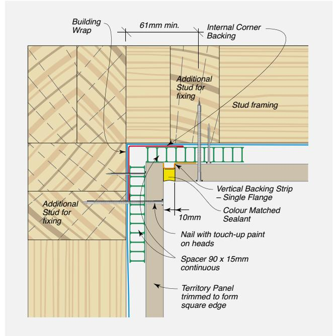
**FIGURE 8.09** External Corner Detail – With Coloured External Corner Trim – Plan View
