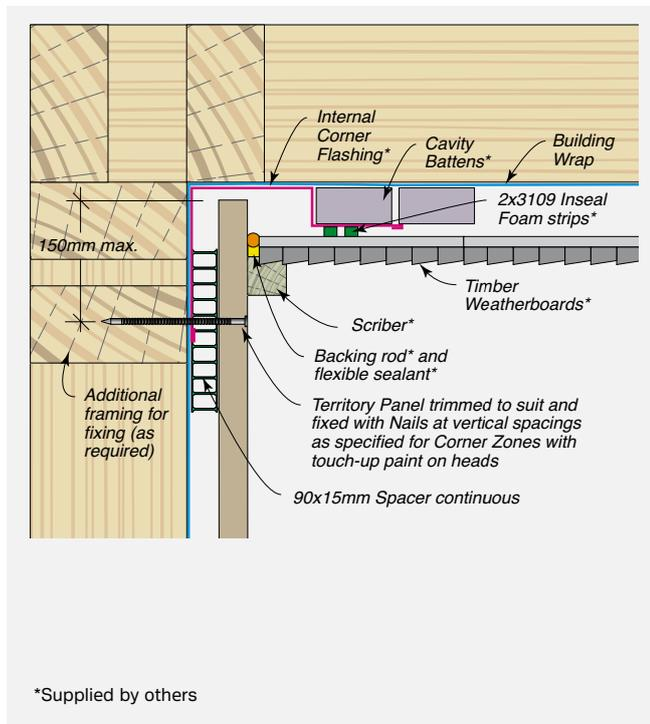
**FIGURE 8.35** Typical External Corner Junction Panel to Weatherboard – Plan View
