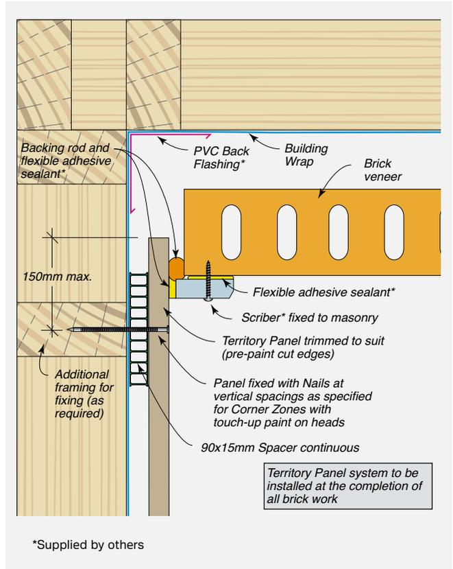
**FIGURE 8.30** Typical Abutment – Panel to Brick Veneer – Plan View
