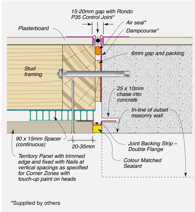
**FIGURE 8.38** Typical Abutment with Direct Fixed Cladding System – Plan View
