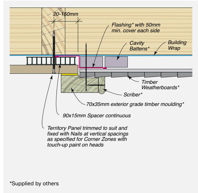
**FIGURE 8.33** Typical Internal Corner Junction Panel to Weatherboard – Plan View
