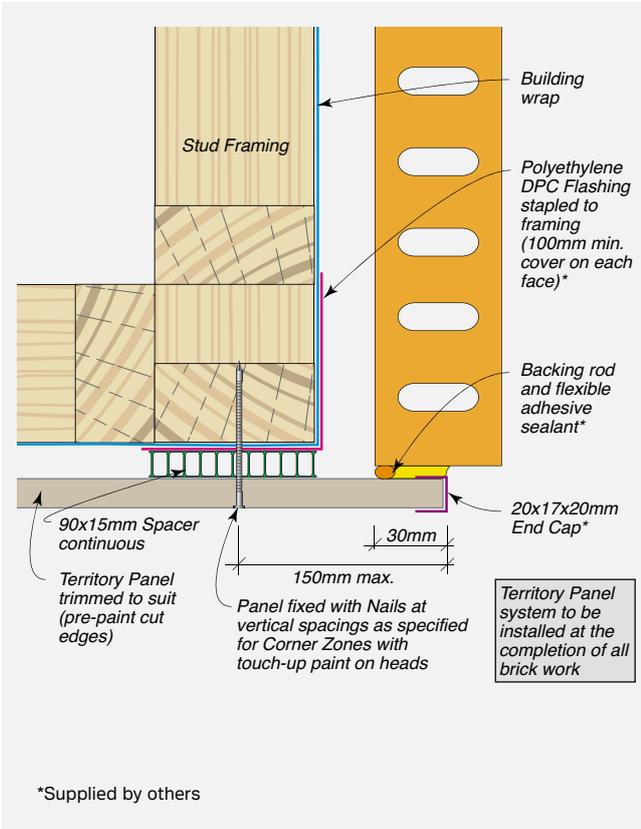
**FIGURE 8.31** Internal Corner Junction – Panel to Brick Veneer – Plan View
