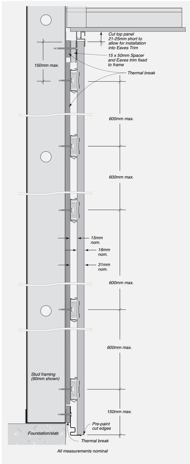
**FIGURE 7.11** Typical Territory System Cross Sectional Detail for Steel Framing where Face Fixing is required – Elevation
