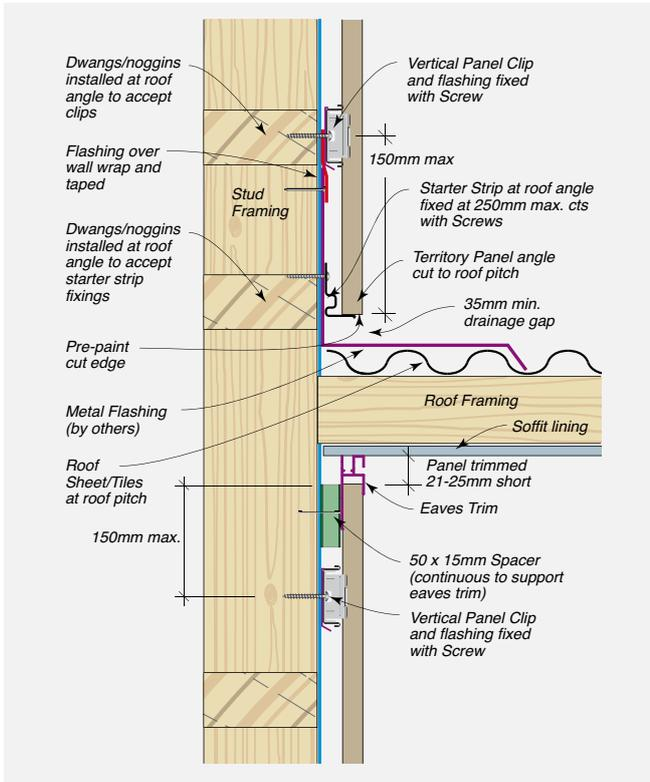
FIGURE 8.23 Junction of with External Roofing
