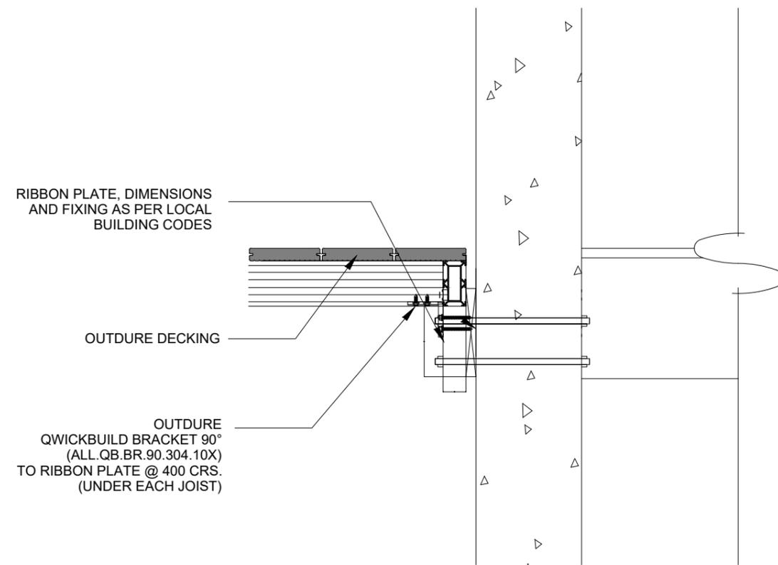
**4 QB-C4 SLAB OR CONCRETE APPLICATIONS**
