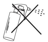
Do not use strong, corrosive or abrasive cleaning materials. Stainless steel surfaces will show scratches if an abrasive cleaning product is used.
