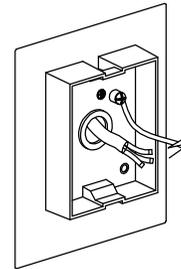
**5** Push the power supply through the cable gland. Affix the rear base to the mounting surface with mounting wall screws supplied. To maintain the IP rating, a round 3 core 0.75mm<sup>2</sup> (min) cable should be used.
