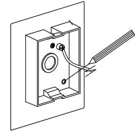
**3** Use the rear base to mark the position of screw holes onto the mounting surface. Use a spirit level to ensure correct orientation.
