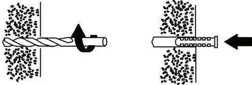
**4** Drill the wall to depth of about 40mm and fit the wall plugs (supplied). Care should be taken to avoid drilling or screwing into concealed electrical wiring/plumbing.
