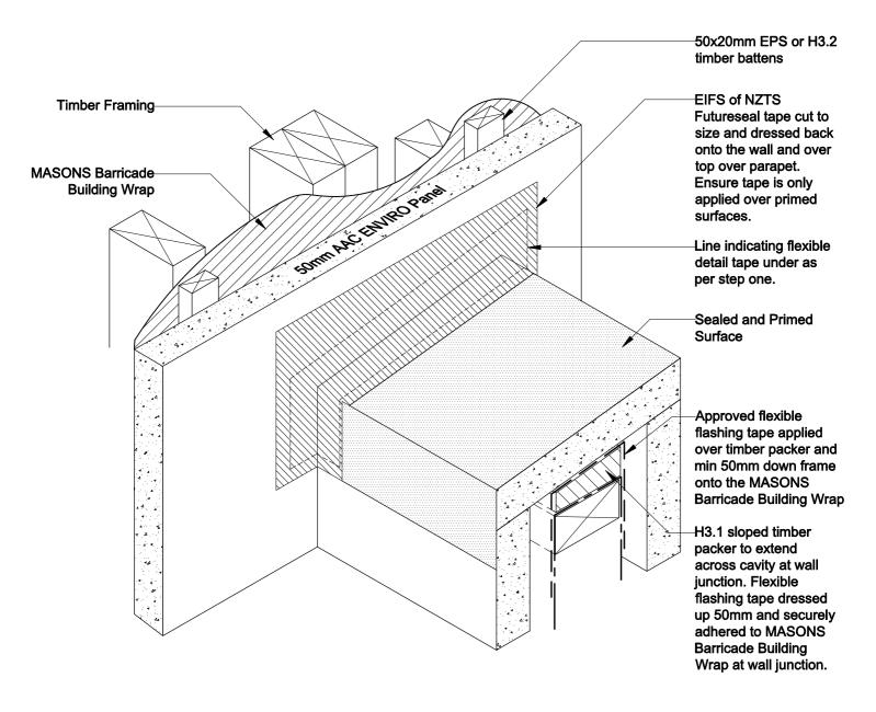
**PARAPET / HANDRAIL** TO WALL JUNCTION **ENVIRO Panel Capping** Step 2
