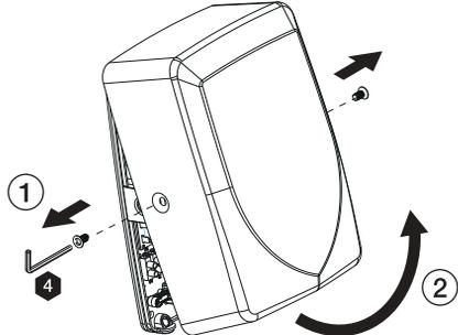
Unscrew front cover from the base of the unit using the hex key provided.
