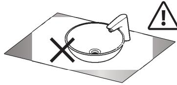
It is recommended to avoid installation of dryer near high reflective objects (mirror, stainless steel washbasins, etc.) in order to avoid errant function of the presence sensor.
