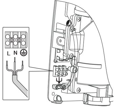
Connect supply and ground wires to terminal block where indicated.
