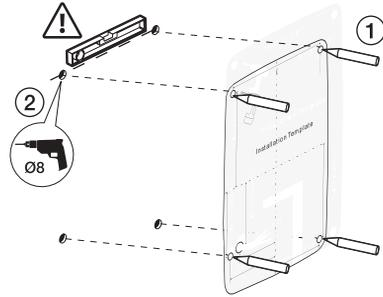
Using the mounting template supplied, mark mounting hole locations for correct height above the floor and drill 4x mounting holes.
