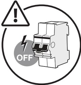
Be sure to break the electric supply before any operation.
