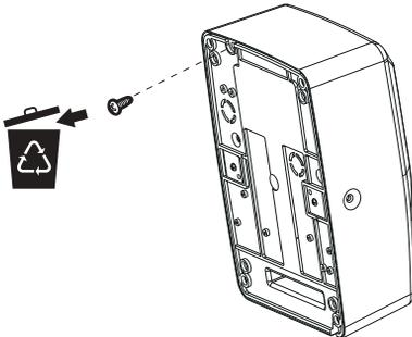
Remove transport screw at the rear of the dryer.
