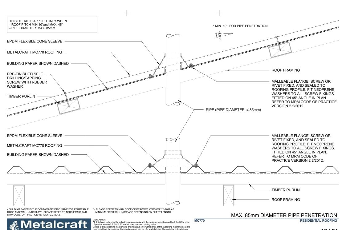
single line for simplicity and is indicative only. Building paper type and method of installation should comply
