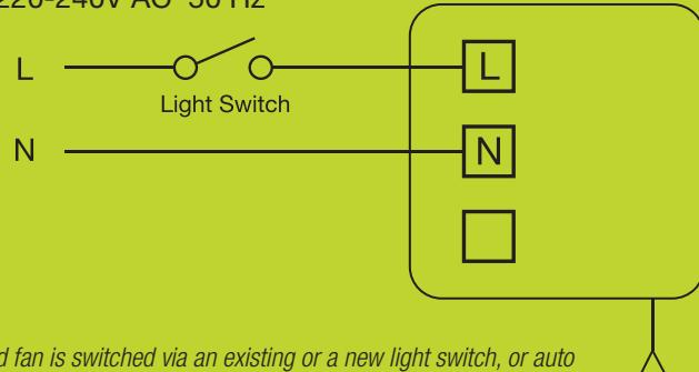
The single speed fan is switched via an existing or a new light switch, or auto sensor, (switch and sensor not supplied) and is controlled by an internal pull cord.
