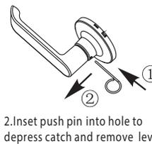
2. Inset push pin into hole to depress catch and remove lever.
