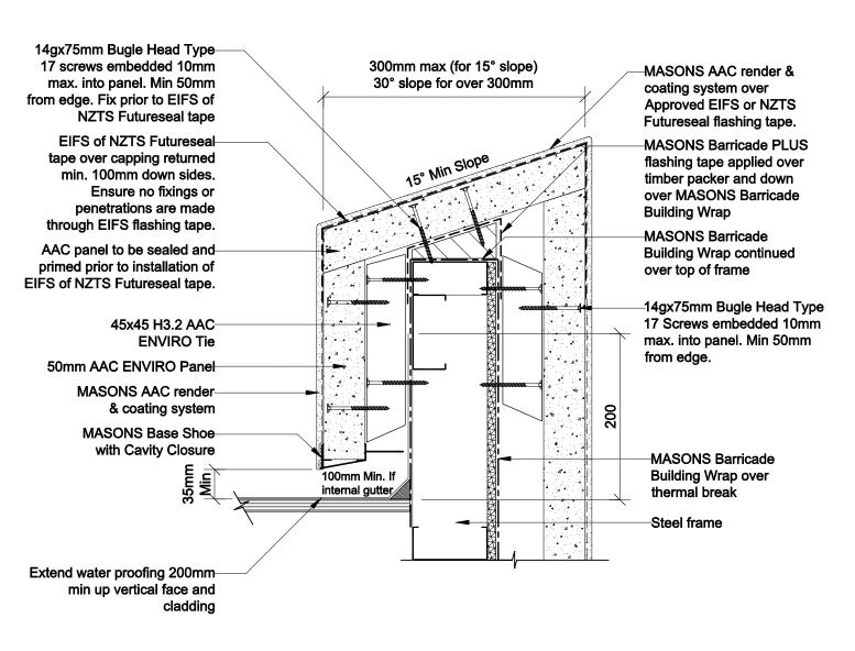
PARAPET CONSTRUCTION -Plastered Capping
