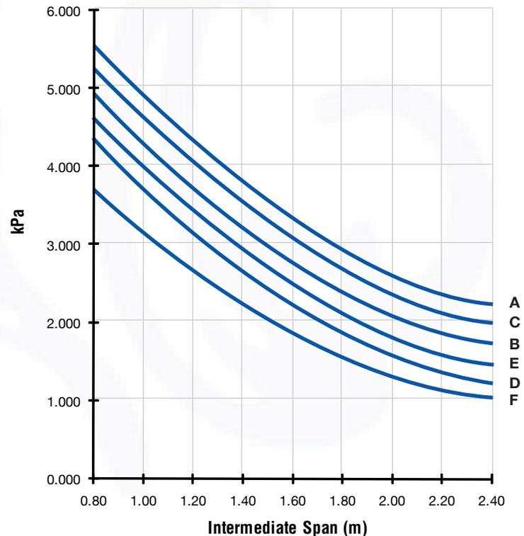
Note: The intermediate spans shown in the graphs above are based on G550 Steel as the base metal. To calculate end spans please multiply the intermediate span calculated by 0.66. Spans are based on restricted access. For alternative metals please contact your local Metalcraft branch.
