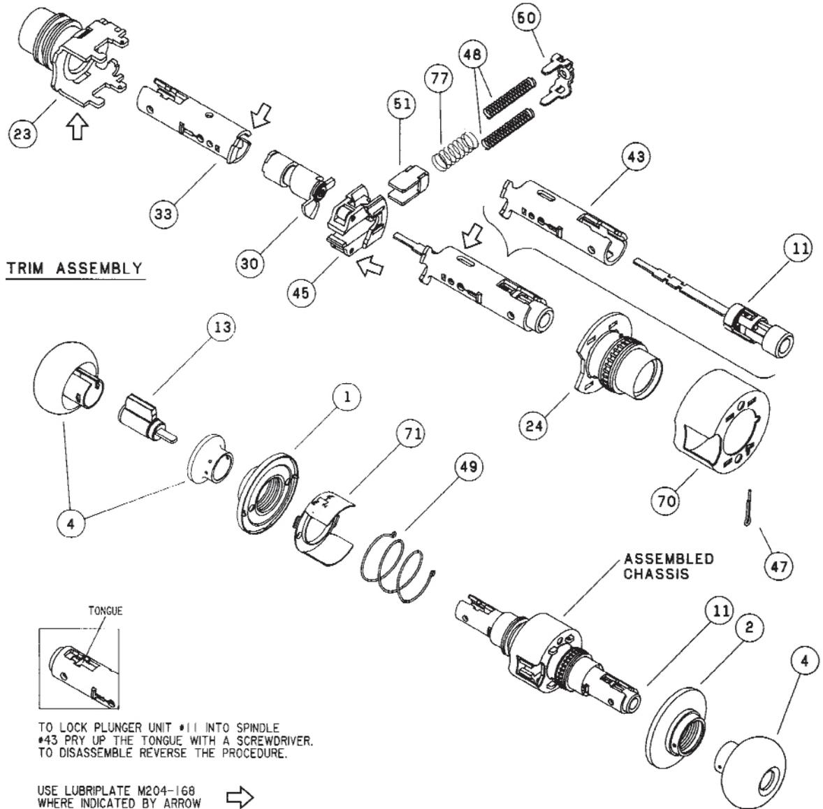
TO LOCK PLUNGER UNIT #11 INTO SPINDLE #43 PRY UP THE TONGUE WITH A SCREWDRIVER. TO DISASSEMBLE REVERSE THE PROCEDURE.
