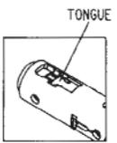
TO LOCK PLUNGER UNIT #6 INTO SPINDLE #43 PRY UP THE TONGUE WITH A SCREWDRIVER. TO DISASSEMBLE REVERSE THE PROCEDURE.
