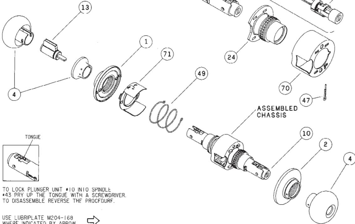
TO LOCK PLUNGER UNIT #10 INTO SPINDLE #43 PRY UP THE TONGUE WITH A SCREWDRIVER. TO DISASSEMBLE REVERSE THE PROCEDURE.
