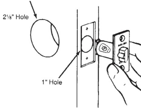
Bore a 1" hole straight into door edge to intersect with center of 2 1/8" hole.
