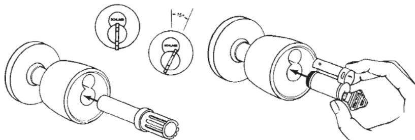
Turn knob over and replace knob on spindle. Slide knob up to knob catch. Insert long end of installation tool into knob until it engages driver. Turn tool one-quarter turn to right, depress knob catch and push knob into position. With control key fully inserted, push core into knob housing, rotate key 15° to the right and insert core completely. Rotate key back to upright and remove control key.
