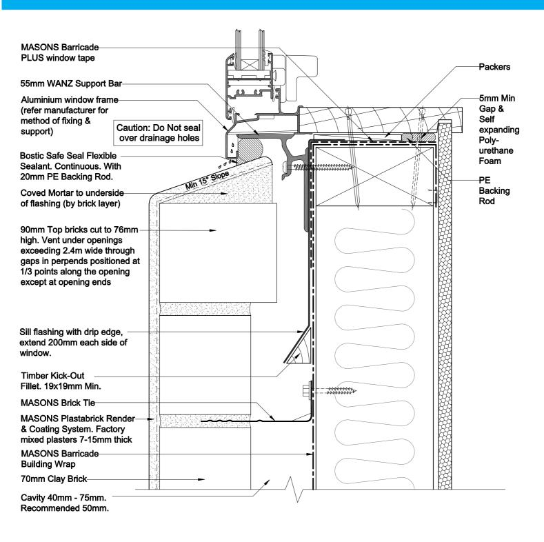
**OPENING FLASHINGS Window Sill - Raking**
