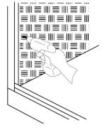
**7.** Apply a continuous bead of silicon to the full length of the channels and waterproofing, indicated by the dark line (inside channel).
