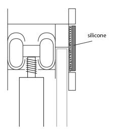
Place the spare detail strip on top of the top track. This will cover the adjustment holes. Do not silicone into place.
