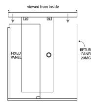
on the fixed panel side and the MG-2W end connector angle will slide over the glass return panel. Ensure the top track is level. Fix the MG-3W end connector bracket to the wall. Tighten the screws into the end connector angle firmly.
