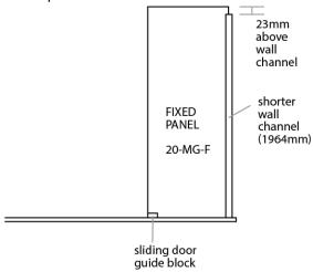
4. Position the glass receiver channel on the base
