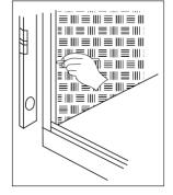
**5.** Apply a silicon bead to the full length of channels. Silicon used must be compatible with anodised aluminium, as well as acrylic or the waterproofing being used.
