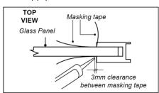
spatula to remove the excess silicon. Remove the masking tape immediately after application.
