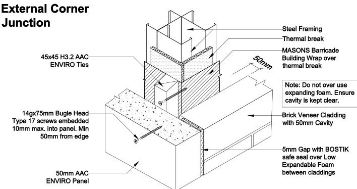
**AAC ENVIRO PANEL / BRICK VENEER External Corner Junction - 3D View**
