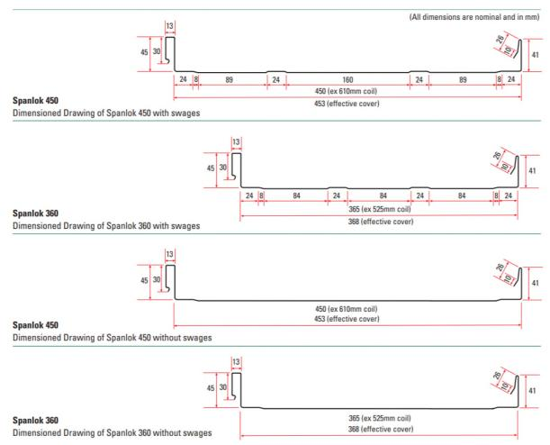
Acceptable Solution E2/AS1 provides for trough profile roofing with a minimum rib height of 38 mm and 210 mm maximum between crests.
