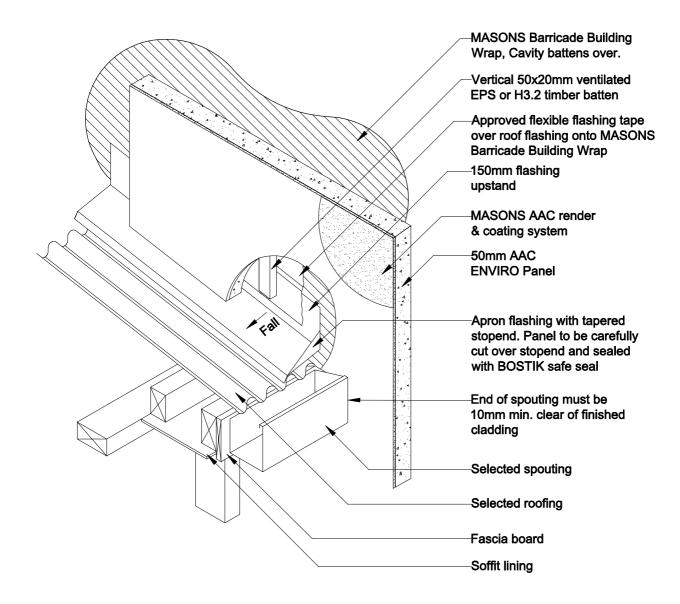
**ROOF/WALL JUNCTION -**KICKOUT FLASHING
