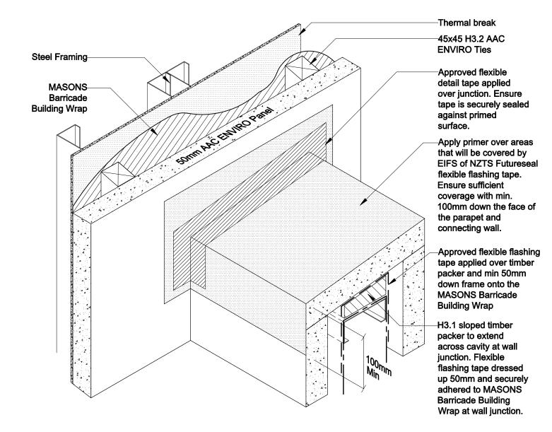
PARAPET / HANDRAIL TO WALL JUNCTION ENVIRO Panel Capping Step 1 **Detail 59 NTS**
