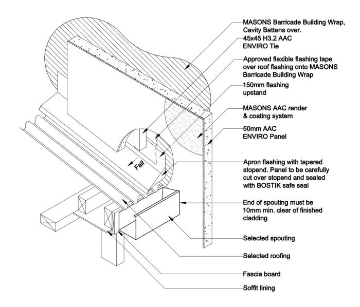
ROOF/WALL JUNCTION - KICKOUT FLASHING
