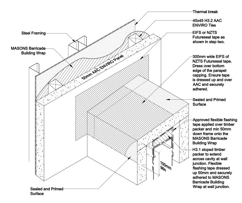
PARAPET / HANDRAIL TO WALL JUNCTION ENVIRO Panel Capping Step 3 **Detail 59B NTS**
