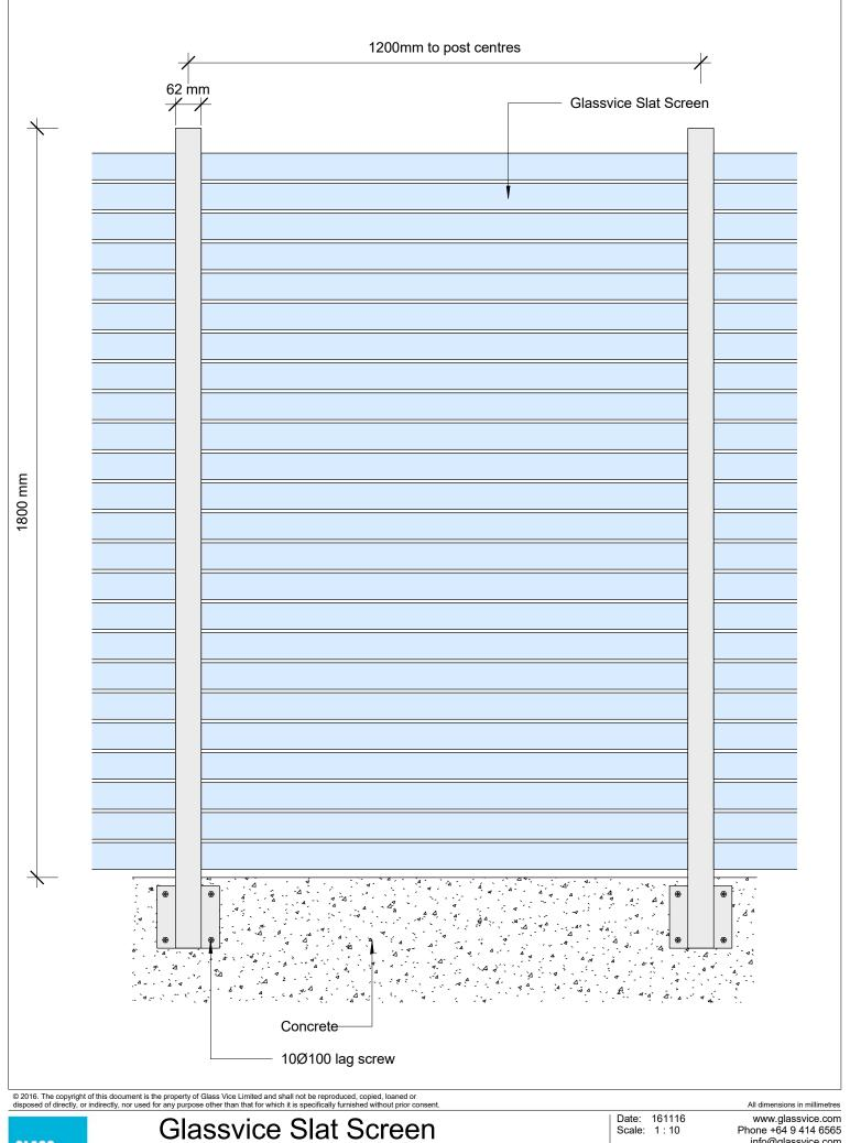
Concrete Side Fix Elevation
