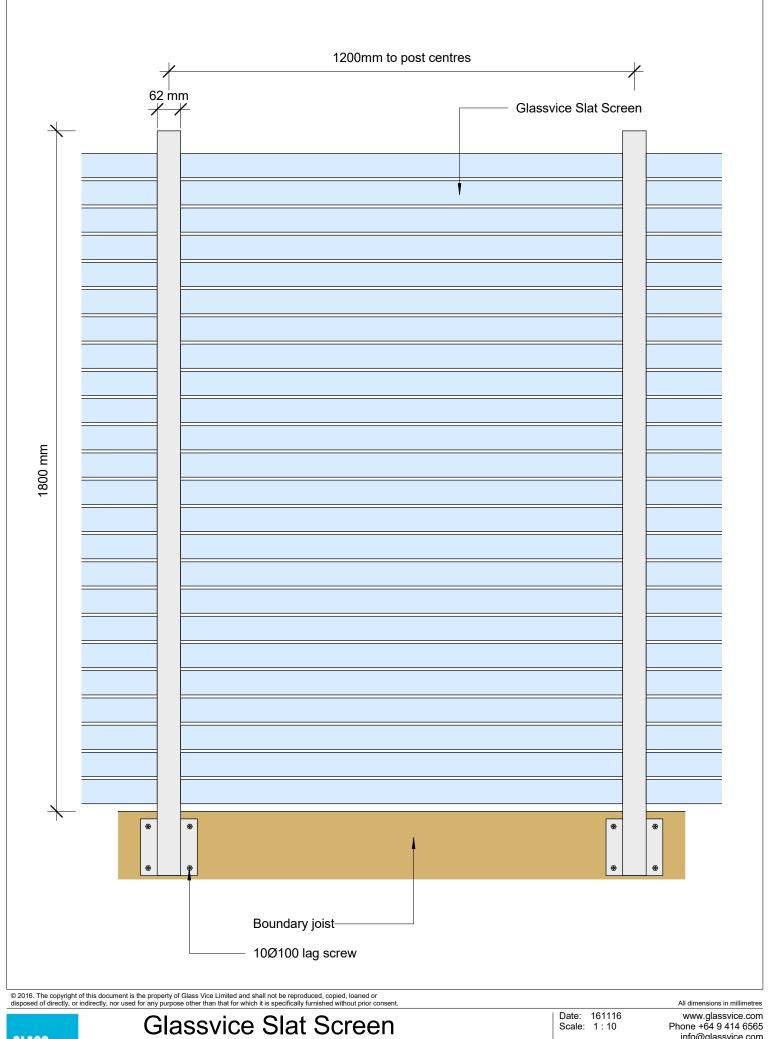
TImber Side Fix Elevation
