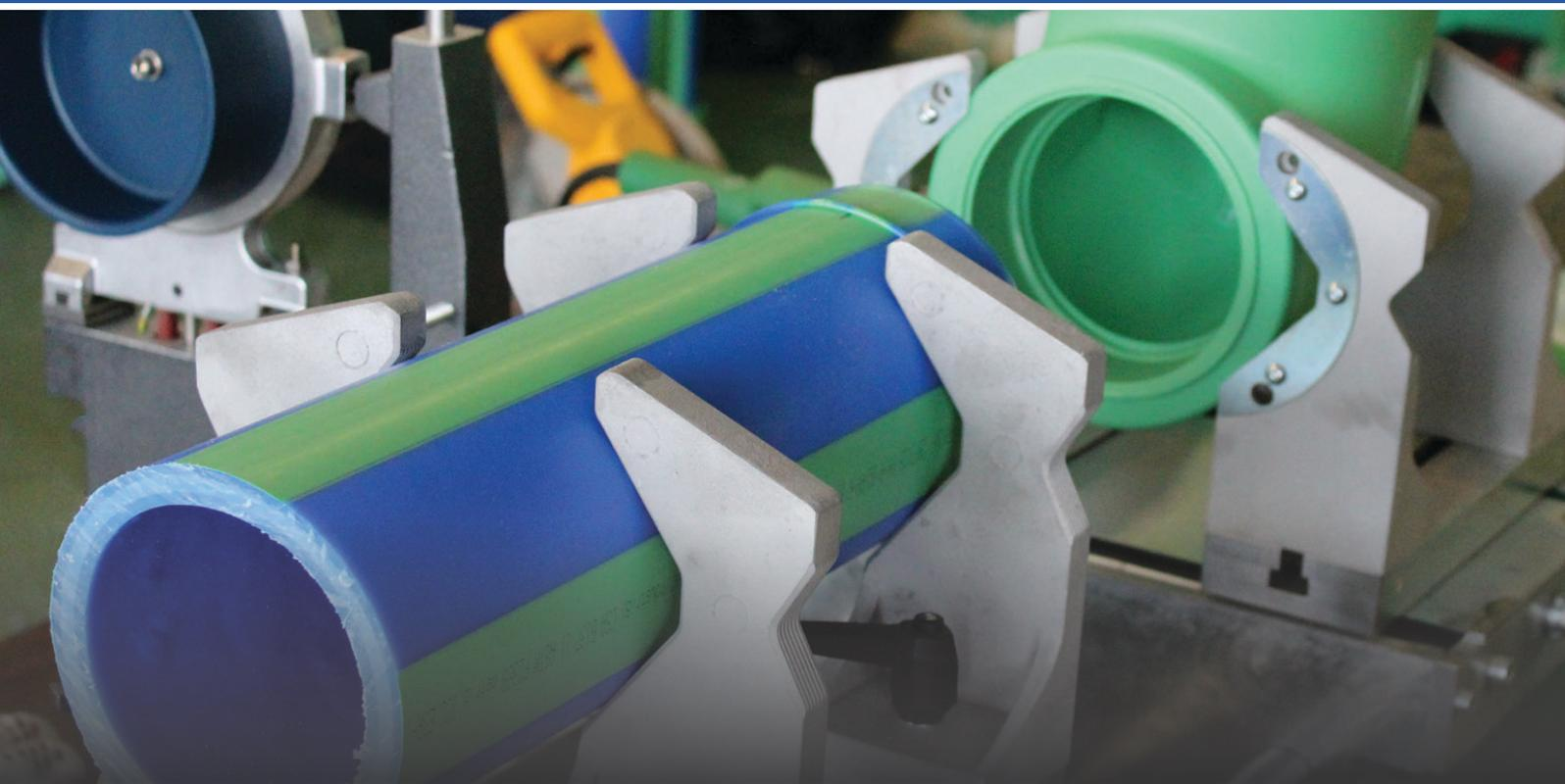
Our hot-water pipes have a reinforced multi-faser layer that reduces expansion by up to 75%.
