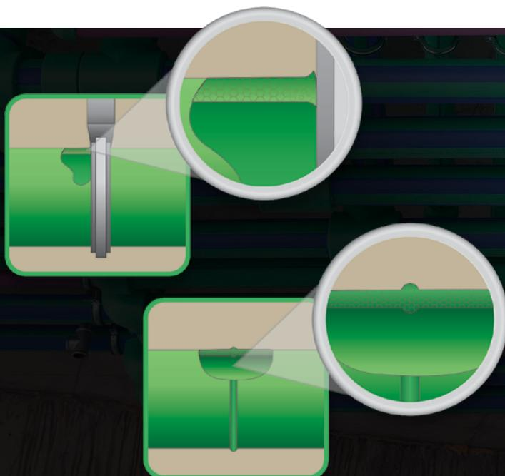
**The heat fusion process takes just a few seconds to make a connection in smaller diameters and only minutes for larger sizes.**
